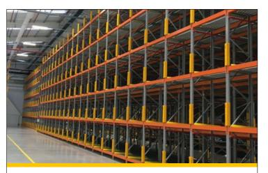
RackGuards can also be installed above ground level to protect racks from loading and unloading damage.
