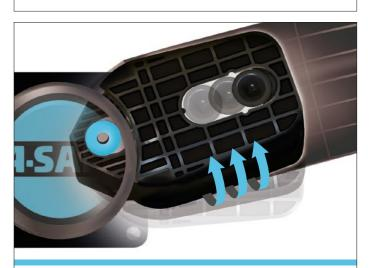
**PHASE 3:** At peak energy, the coupling twists further, engaging the post pin and instigating torsion of the post to dispel remaining forces.
